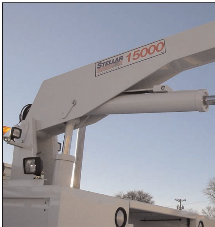
The crane MUST be in the stored position before transporting.
