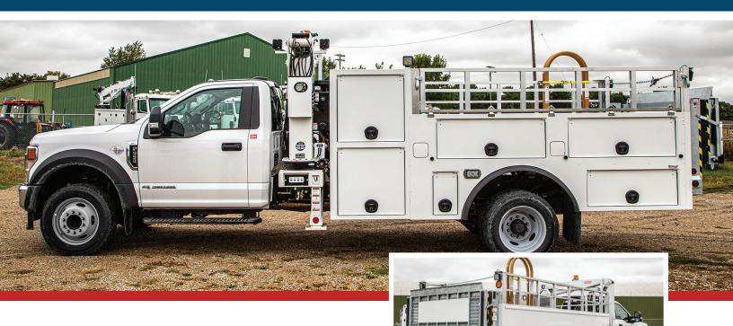
The Stellar 1184-13 Mini OTR is without a doubt one of the most popular trucks in the commercial fleet service vehicle line-up. Its versatility comes from the combination of service body, tire handling crane, tire loading liftgate, and a large hydraulic-driven air compressor. The crane will handle up to a 4,000 lb. OTR tire as well as large agricultural tires. This package provides 4,000 lbs. of payload to haul approximately twenty-two (22) truck tires or up to two (2) 29.5x29 OTR tires.
