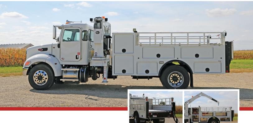
The Stellar 1184-15 AG offers several of the same features of the 1184 with the addition of 3-feet of cargo area. The Stellar 1184-15 AG is designed to fit a 26,000 GVW and larger chassis with a minimum of 144" CA. The combination of a larger service body, tire handling crane, tire loading liftgate and a large hydraulic-driven air compressor, makes the 1184-15 AG a very versatile and productive service unit.
