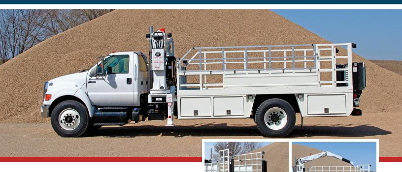
The 138-15 Mid Size OTR is the service truck of choice when the Mini OTR is not quite large enough. The body comes in either a 15-foot flatbed or with a 15-foot rack body with over 60 cubic feet of storage for a combination OTR, fleet and AG service vehicle. The 6000 series crane will handle up to and including the 45/65x45 OTR tire. This package provides 8,500 pounds of payload. The 15-foot rack body will hold approximately forty (40) large truck tires.
