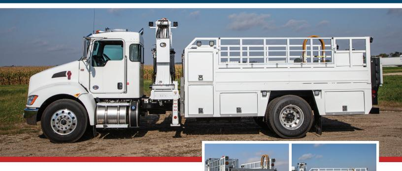
The 138-215 Mid Size OTR is the service truck of choice when more storage is needed. This package provides provides 8,500 pounds of legal payload. The 6000 series crane will handle up to and including the 45/65x45 OTR tire. This package provides 8,500 pounds of payload. The 15-foot rack body will hold approximately forty (40) large truck tires.
