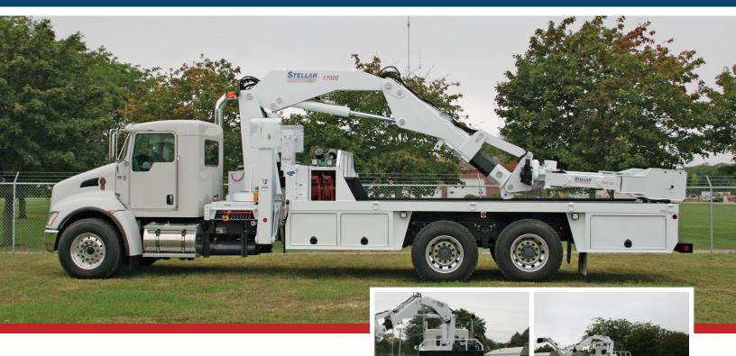
Designed from the ground up to provide maximum lifting performance and solid stability, the Stellar® 17000 is the largest OTR crane in the industry allowed on a single axle truck. It also offers over 18' of stabilizer spread to keep your truck stable.
