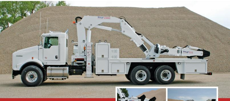
The Stellar 23000 OTR series tire service crane fits the need of OTR tire service technicians who need well rounded versatility. The 23000 OTR series is the one to turn to when you need a reliable and dependable service truck. The 315-degree crane rotation is carried out through a turntable bearing with a high torque planetary gear reduction system. The hexagon-shaped secondary and extension substantially increase boom strength over competitive square-shaped booms, ensuring solid performance.
