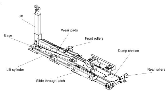
Base section The base section of a Stellar Slider may also be called a sub-frame. All Stellar Slider hooklifts are
